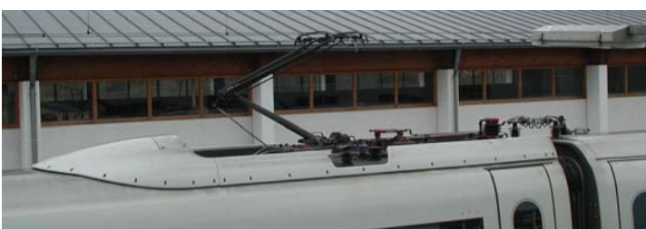
left: figure 6: pantograph with shroud and current wire; right: figure 7: roof antenna
